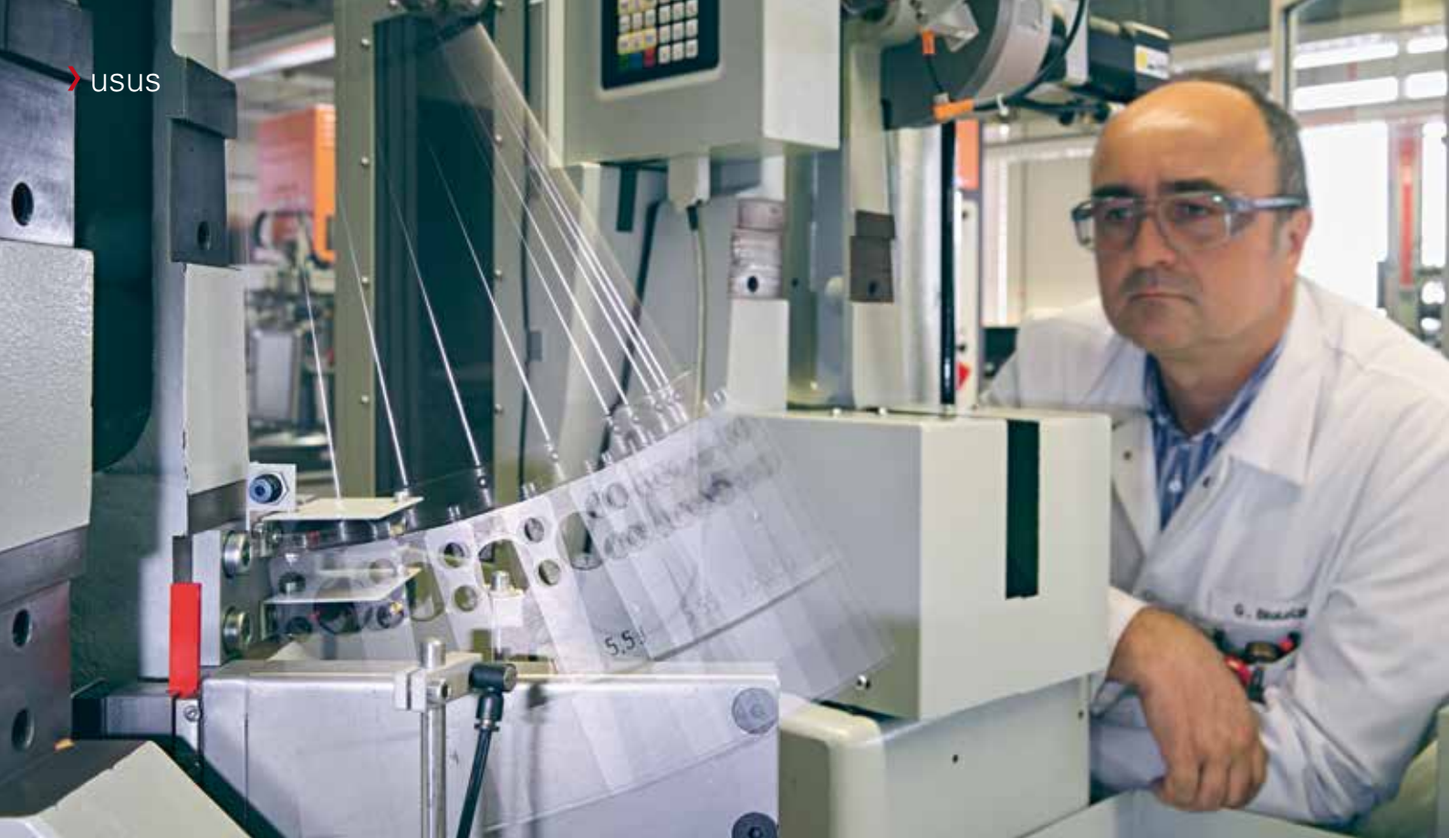
The Charpy impact test in accordance with the IZOD standard provides information about the deformability of a plastic
