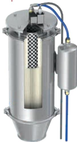
with a pulse of compressed air that blows trapped ingredient back into the process. In a continuous process, jet filter cleaning occurs at the end of the refill during the material stabilization phase without interfering with the gravimetric cycle. When very expensive or toxic materials are involved, a jet filter is a must, but it can also be a good option for other powders and fine pellets. "The best
