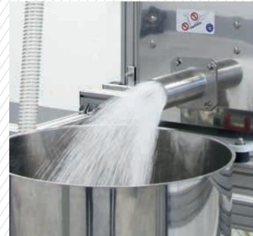
Img. 4: Vented air pushes ingredient out in the event of a blocked filter
