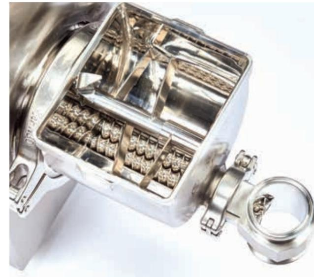
Different screw profiles can be used depending on which ingredient is being fed.
