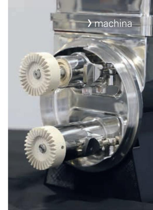
*No edges, corners or undercuts: the hygienic design of the DDSR20 enables rapid cleaning.*
