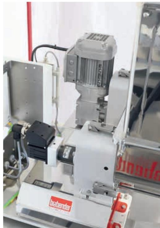
*The three-phase motor (rear) and the new servo-smart motor*
