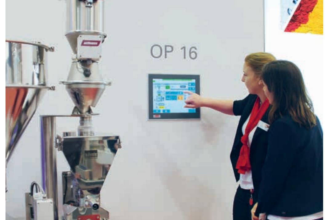
*The existing proven OP 16 operator interface now has the capability to control feeder refill via a vacuum conveyor process.*
