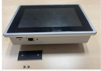
Step 3 Unlock the Micro SD card by applying light pressure (spring mechanism) and then remove it
